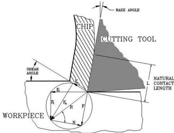
Figure 3. Graphical depiction of three systems of orthogonal forces in chip formation.
