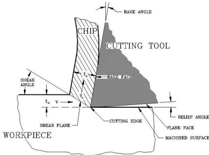
Figure 1. Idealization of orthogonal machining showing the basic geometry of chip formation on the shear plane.
