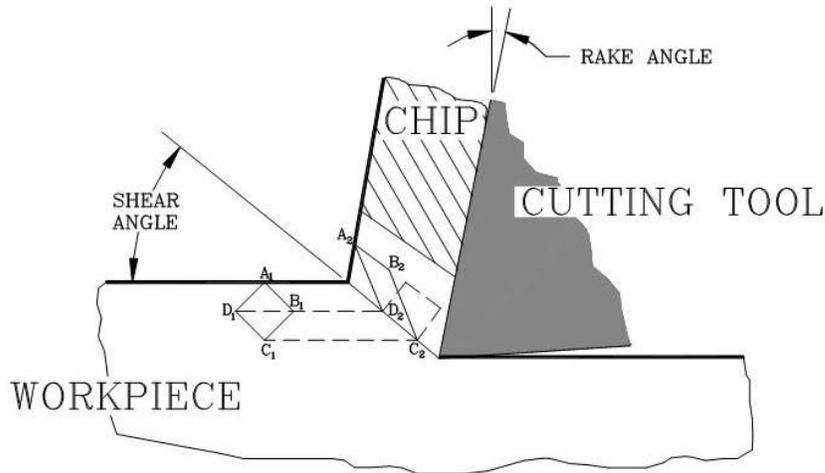
Figure 2. Graphical depiction of the strain of element ABCD as it moves through the shear plane, defined by the shear angle.
